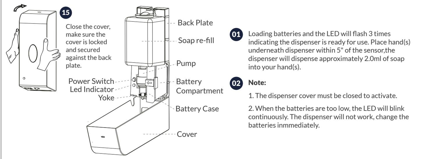
**15** Close the cover, make sure the cover is locked and secured against the back plate.
