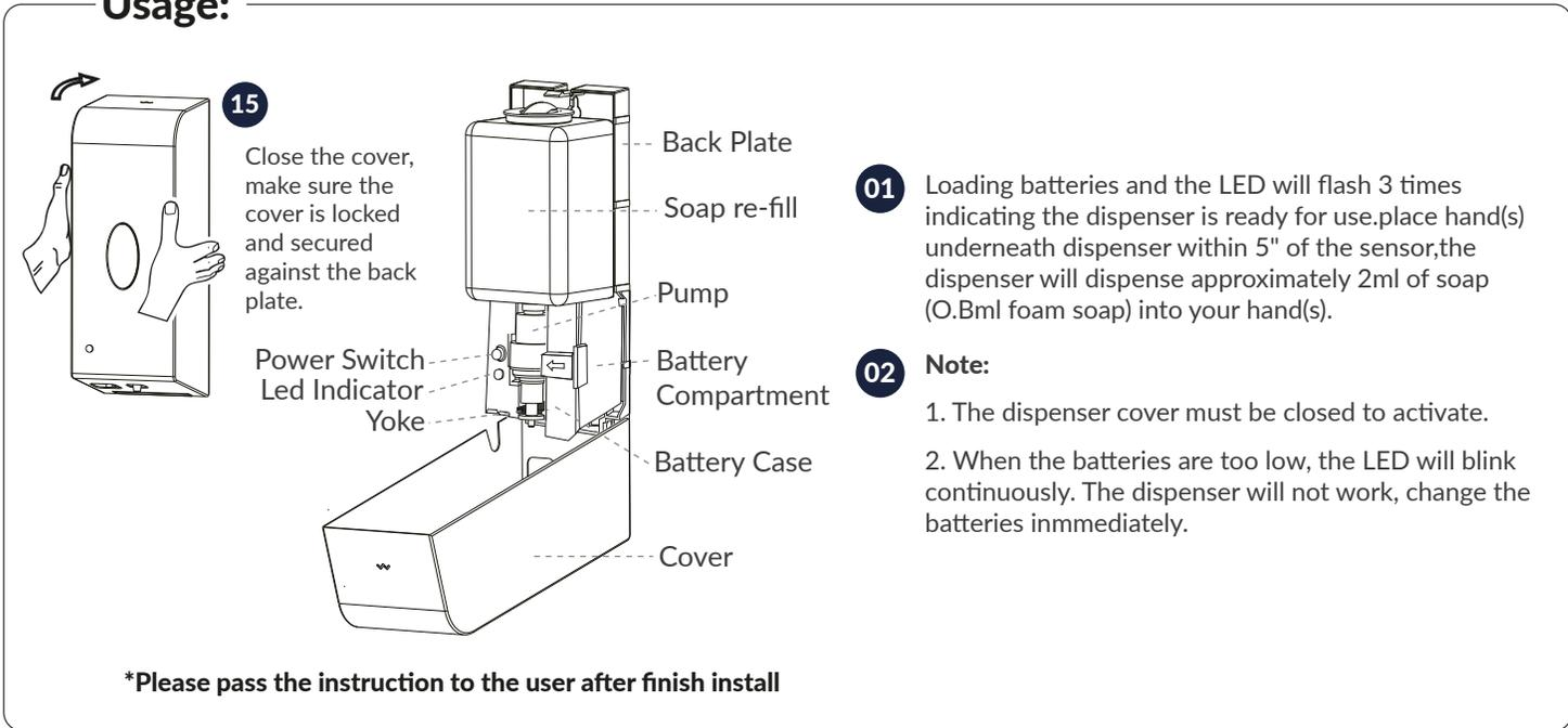
**15** Close the cover, make sure the cover is locked and secured against the back plate.
