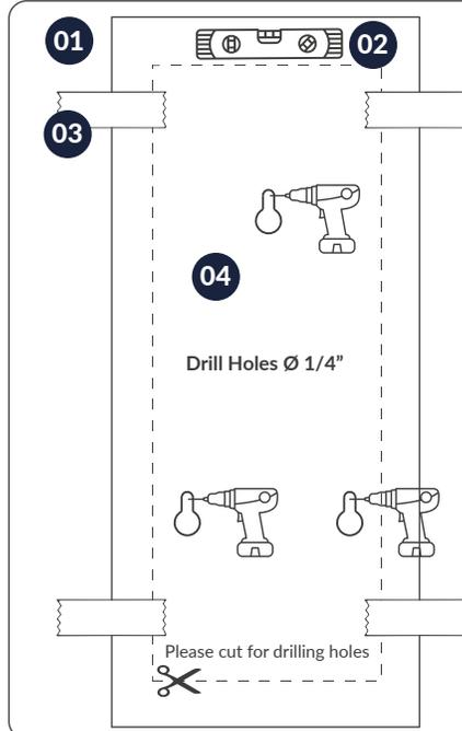
Once the location for the Soap dispenser has been decided, proceed with the installation steps below, if the soap dispenser is installed above the sink, leave a space of 18" from the top of the sink to the bottom of the soap dispenser as shown below in figure (A).
